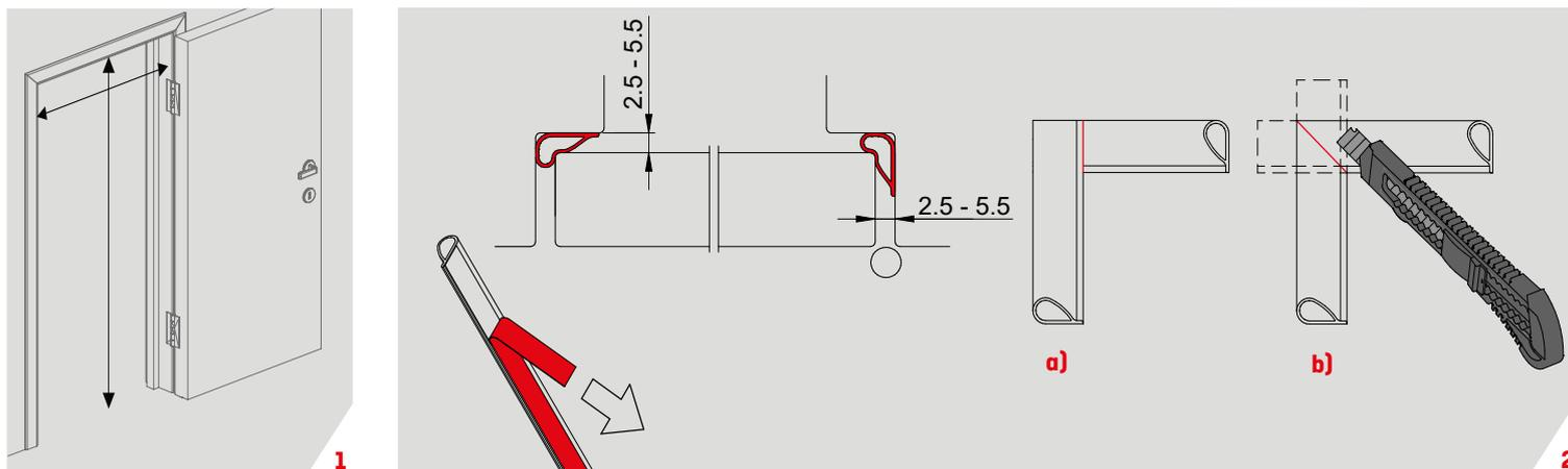
**1** To be fitted with the door fully opened. Stop and face of the frame must be dry, dust and grease-free; clean with isopropyl alcohol. Measure the height and width of the door frame and cut the seal to the appropriate length.
